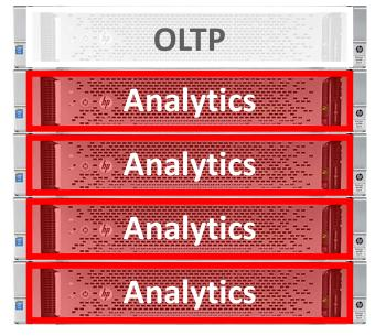
5x Latest Generation HP DL380 10 chips, 180 cores RHEL
